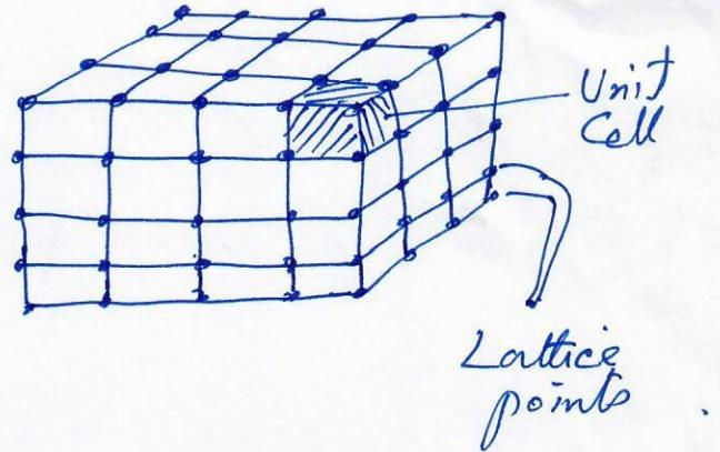
There are 14 - types of unit cells or Bravais lattices in seven crystal structures.
